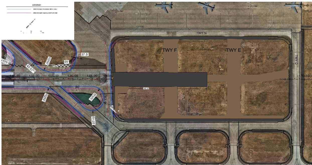
Figure 2-2: Proposed extension of overrun on the 21R end of 21R03L, showing excess taxiways removed.
