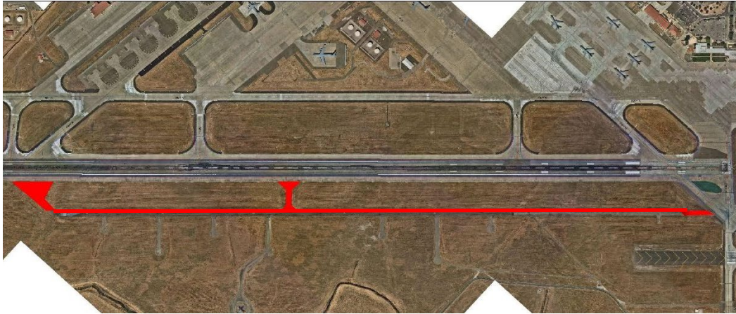
Figure 2-4: Excess pavement proposed to be removed (highlighted in red) and converted to turf
